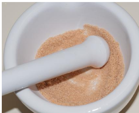
Figure 6: The Amberlite resin is pulverized in a mortar © Centre de Conservation du Québec
