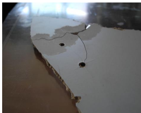
Figure 7: Overflow of epoxy on the outside of the back corner piece after the first gluing.
