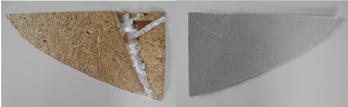
Figure 11: Front corner piece inside and outside after repair.
