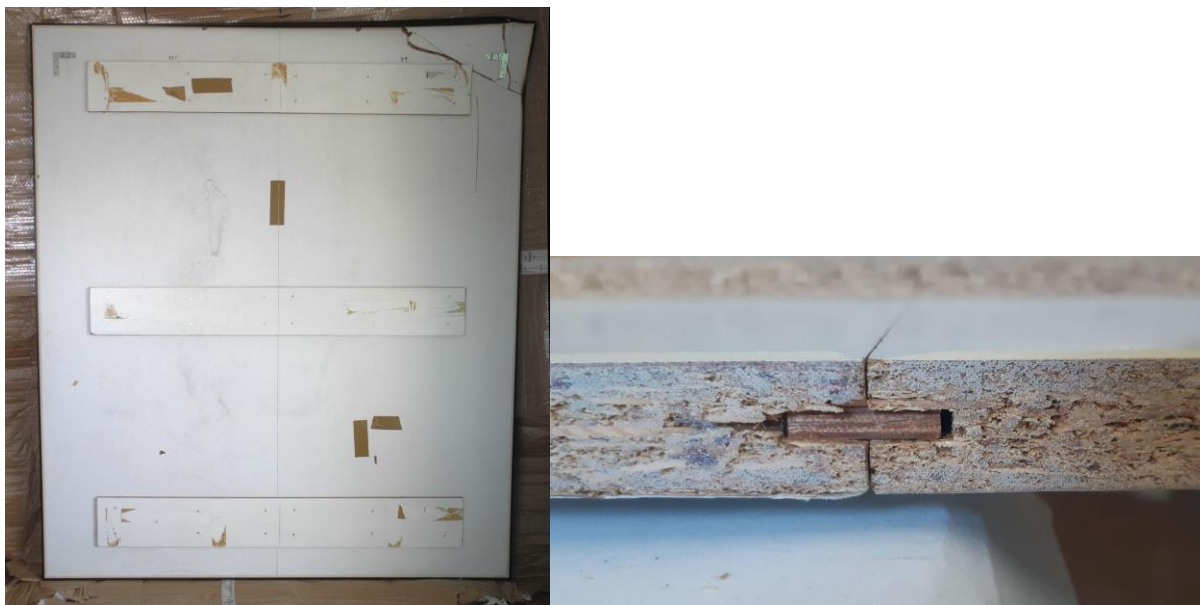
Figure 1: Artwork's verso and loose tongue and groove joint (top edge, panel's intersection)
